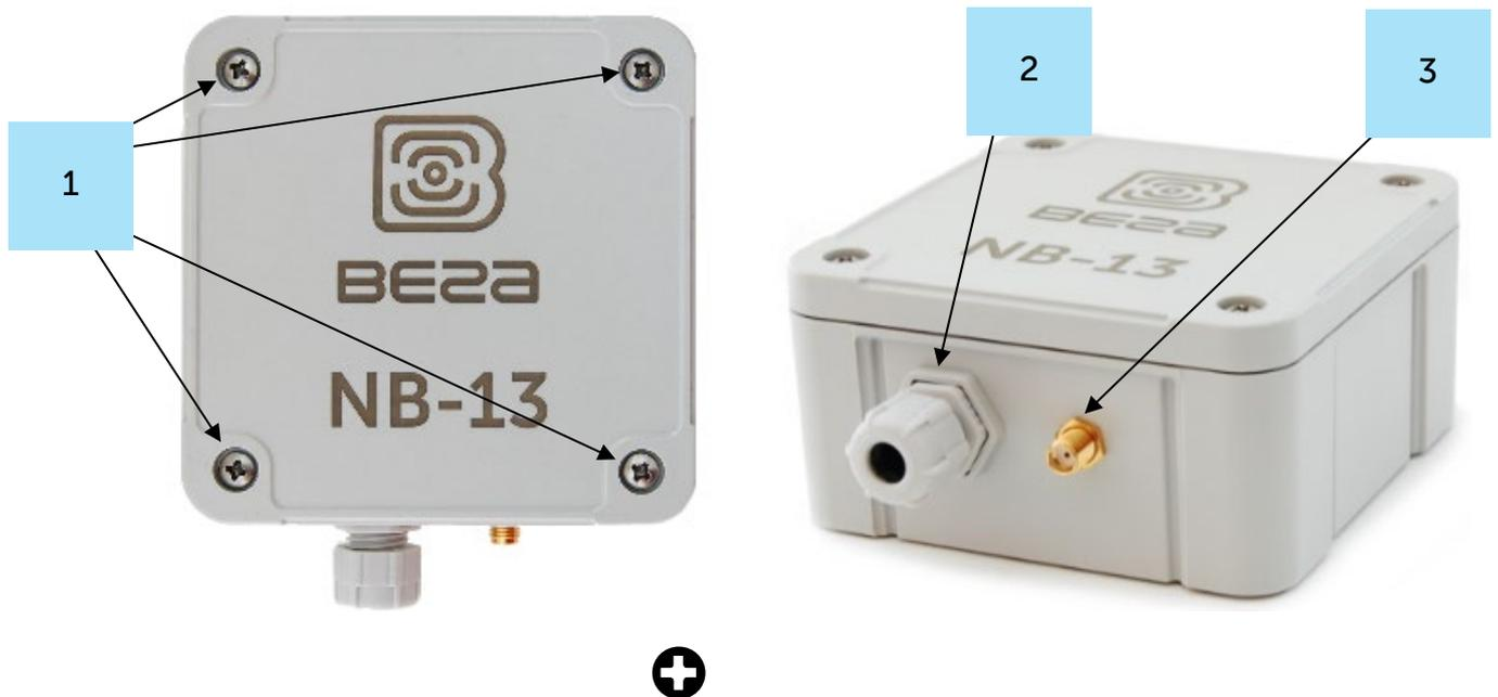
2 – cable gland of M12 size for installing the cables and wires with circular cross-section with a diameter of 5...6 mm
